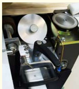
precision glue application, adjustable to veneer species and throughput speed
