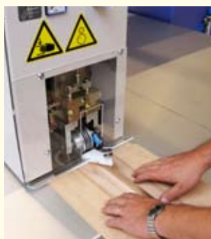
optic-controlled automatic infeed for efficient charging
