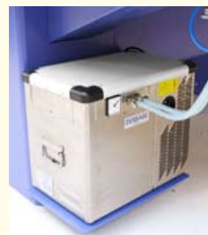
integrated glue pot cooling allowing for extended glue lifetime
